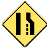
Lane Ends, Merge Left
