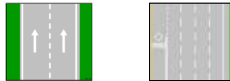
One direction roadway, passing permitted One direction roadway, separating express lane or carpool lane from general lanes—crossing prohibited
